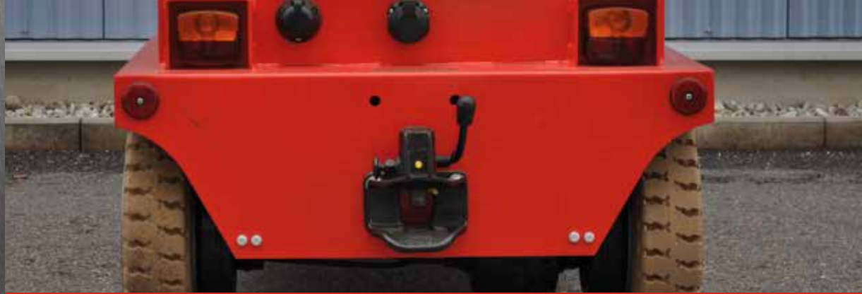
Model 712: Light B, automatic mirror, trailer coupling, light super-elastic tyres
