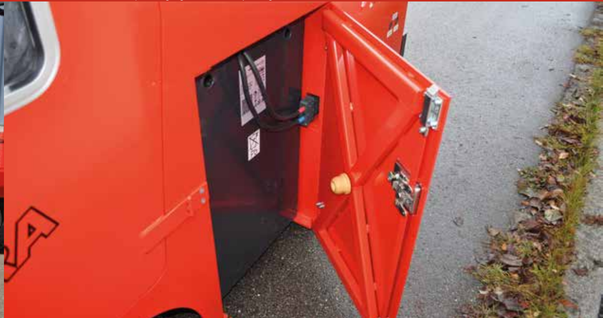
Model 720: Quicker battery changing via lateral opening in the frame
