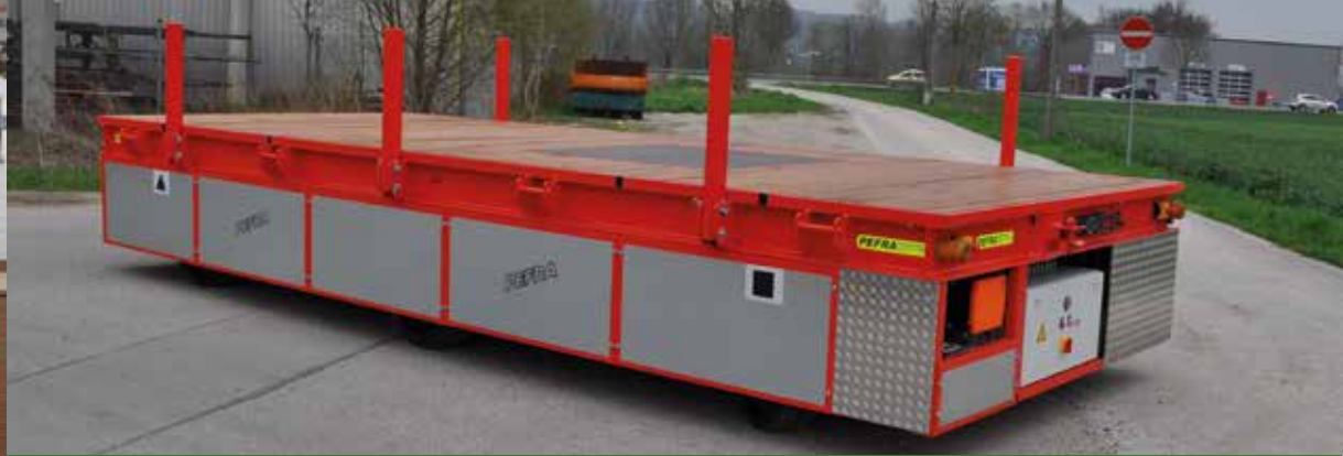
EGW: 20 t, steel pipe transport (up to 18m)
