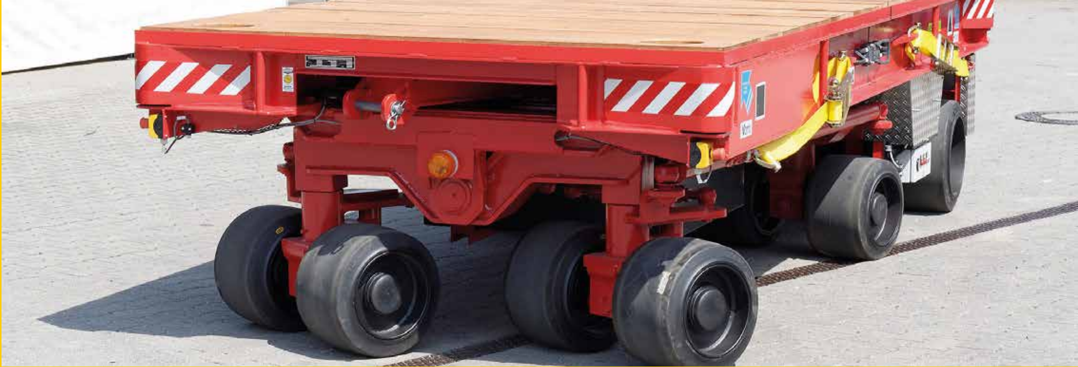
EGW: 42 t with swap bodies, transport of forged billets
