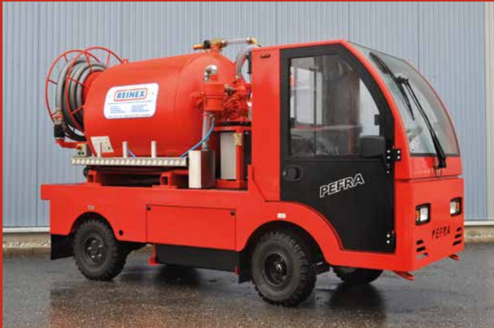
Model 625: Hygiene services in confined spaces - specialist model with suction unit
