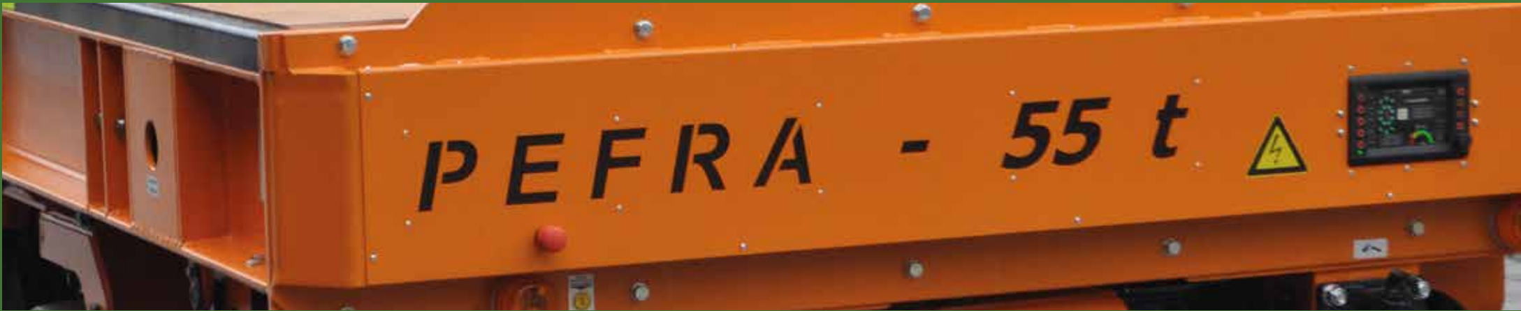
Model 40784800 EGW: 55 t, forming die transport
