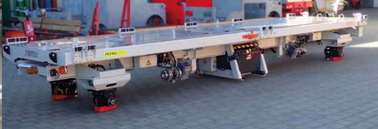
EGW: 2 t, transport of client-specific boards (mould carriers)
