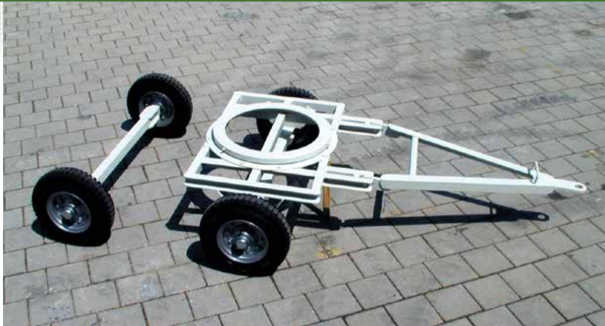
Heavy-duty undercarriage: 2 t
