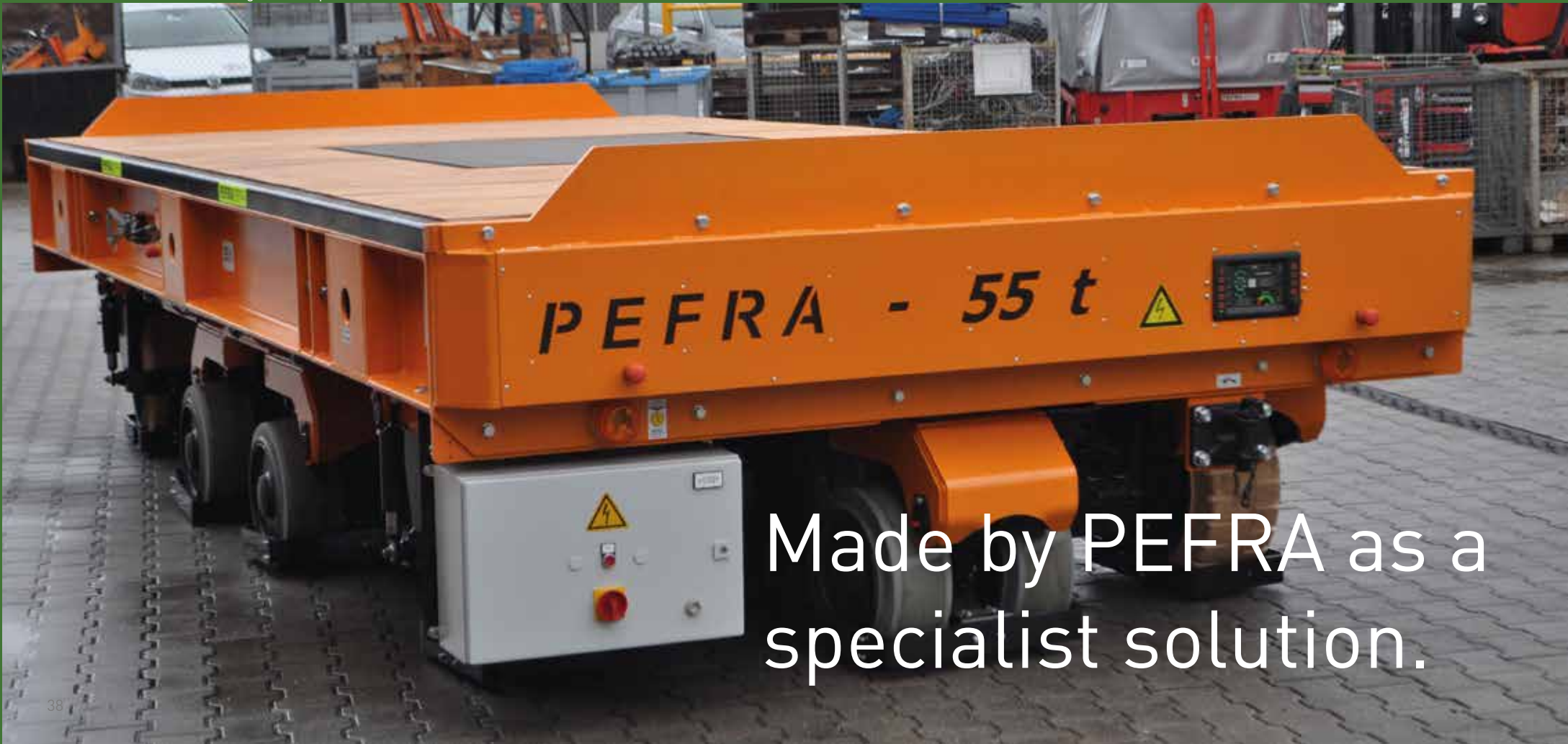
Model 40784800 EGW: 55 t, forming die transport
