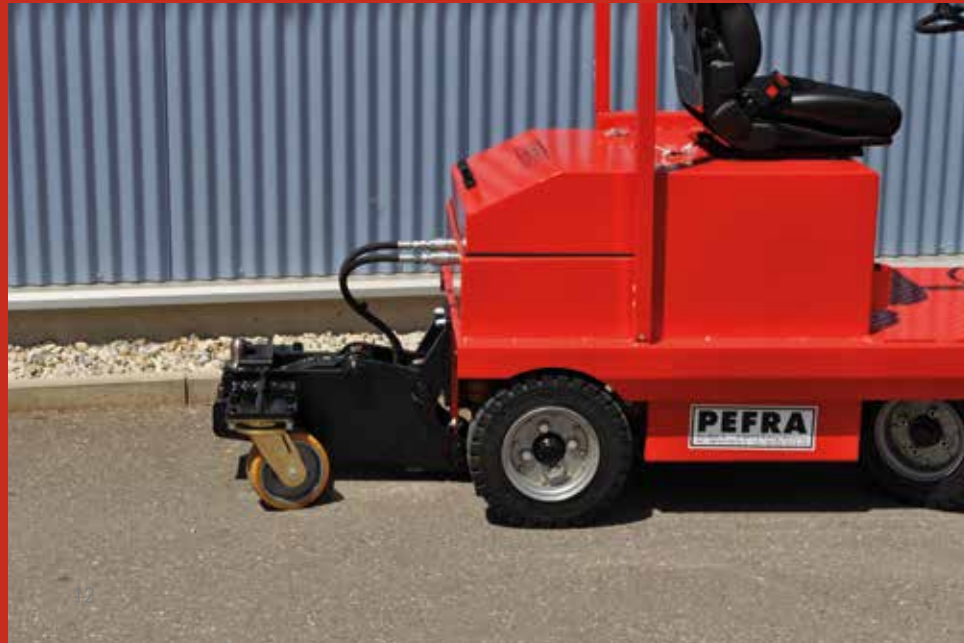
Details: Bright internal lighting and sunroof in accordance with German Road >traffic Regulations Model 712 rolling pallets: Pallet capture - without dismounting, yet precise and quick
