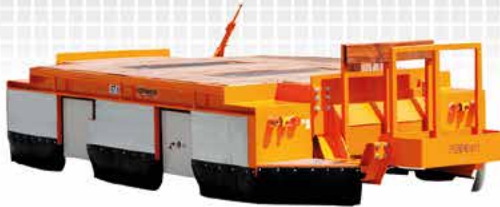
Designation: EFW Payload/speed.: 57 t/4 km/h
