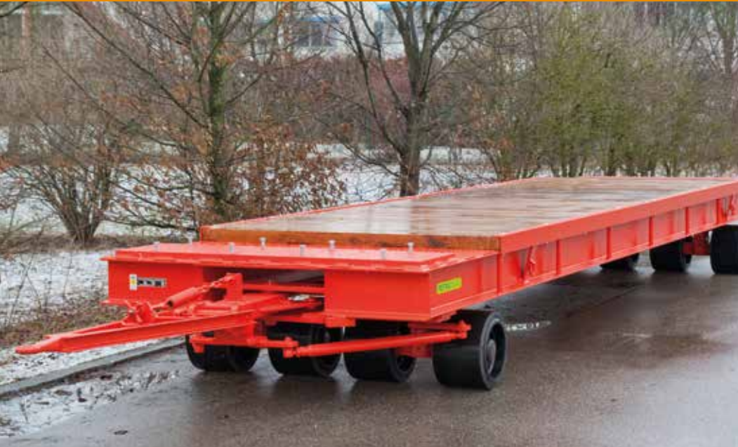
Platform with rotatable seat for the heaviest of chassis Trailer for transporting paper reels
