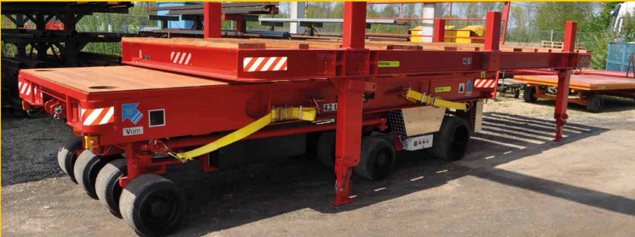
EGW: 42 t with swap bodies, transport of forged billets
