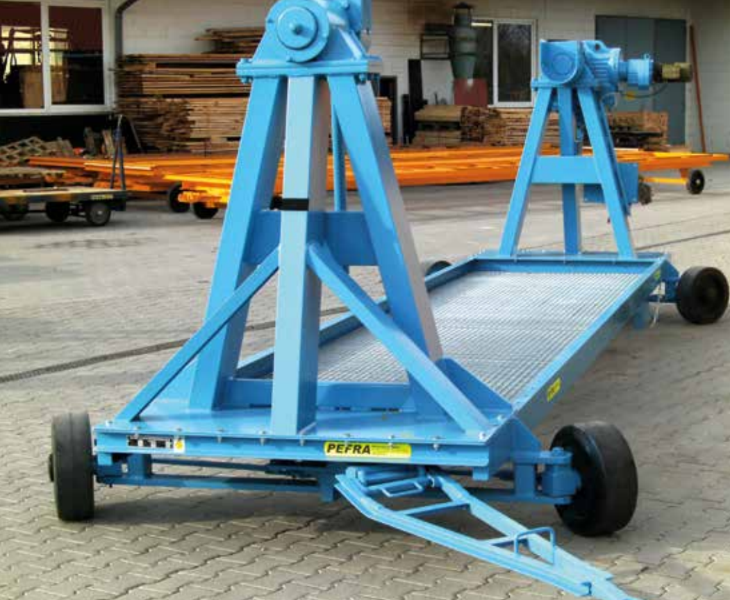
Platform with rotatable seat for the heaviest of chassis Trailer for transporting paper reels
