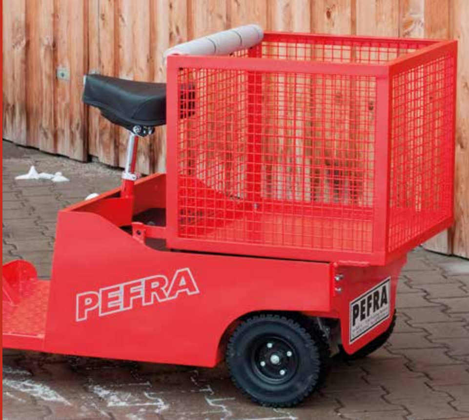
Model 505: With tipping cage and dumping function
