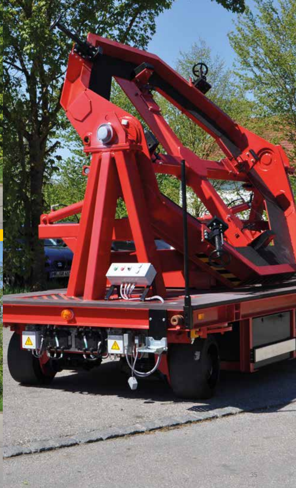
EGW: 15 t, transport of gear rings
